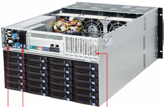
①. Redundant power supply or Standard 2U Power Supply ②. 2*2.5" HDD/SSD ③. PCI/PCIE Expansion Slots
